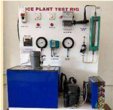
Ice plant test rig
